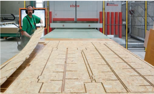
The 5-axis system with nesting function can process formwork panel material measuring up to 6,000 x 2,500 mm.
