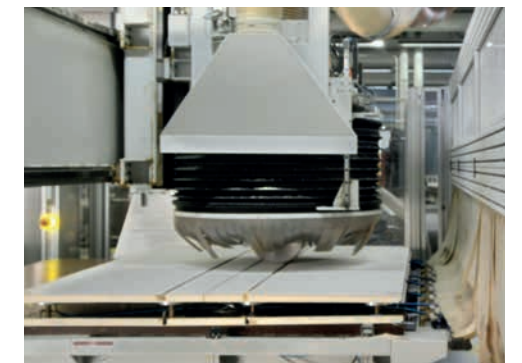
Cutting of components with a 250 mm saw blade: In the process, two components made according to the same production and construction method are manufactured synchronously to achieve a higher output.
