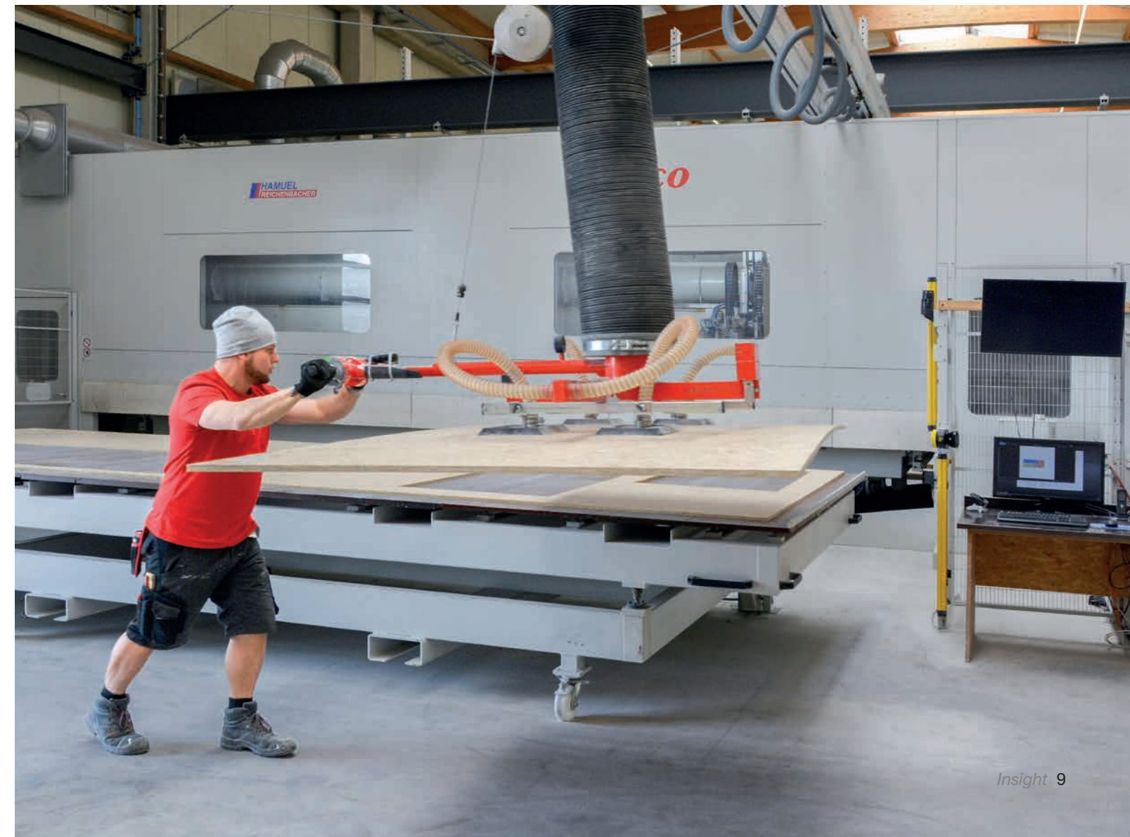
The operator can lift nested plates from the removal table.
