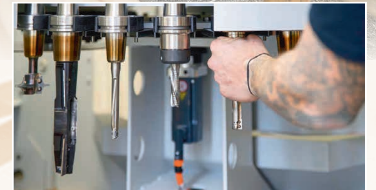
The tool magazine with its 15 places is sufficient for the majority of the machining operations.
