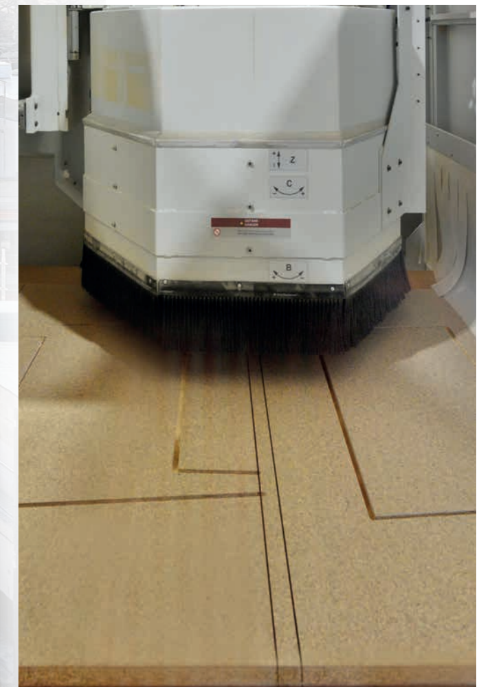
Cutting of cap formwork: precise and quick milling of the templates from the panels.
