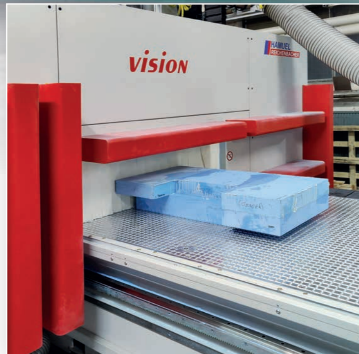
The VISION-II at the beginning of milling the blanks for the monocoque.
