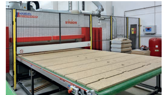
Discharge table with conveyor belt for components and waste.
