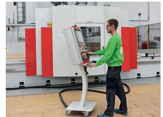
Daniel Scheuber operates the 5-axis machining centre with nesting function by means of a modern Siemens control system.
